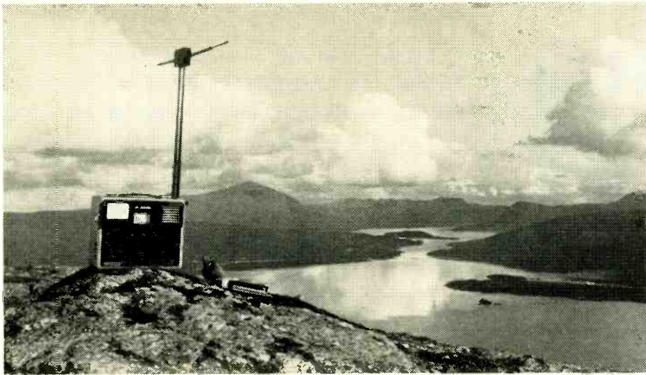
Fig. 4. Field-strength measurement during the route survey.
