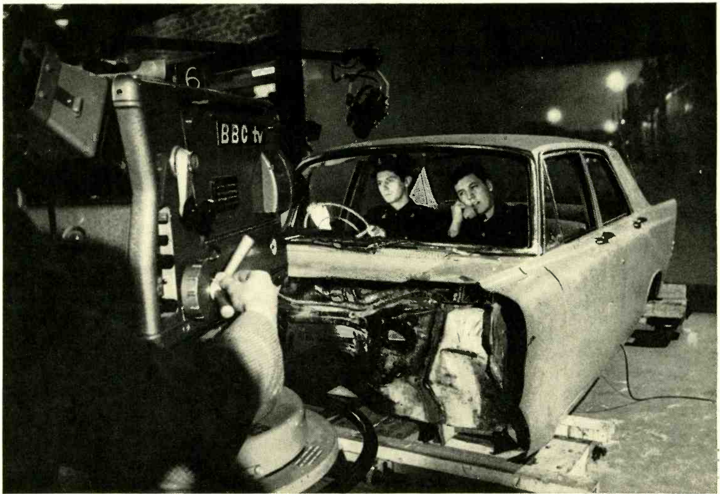
Fig. 1. A mock-up of a Crime Patrol car being shot against moving back projection during a rehearsal of a "Z Cars" episode The Listeners .
