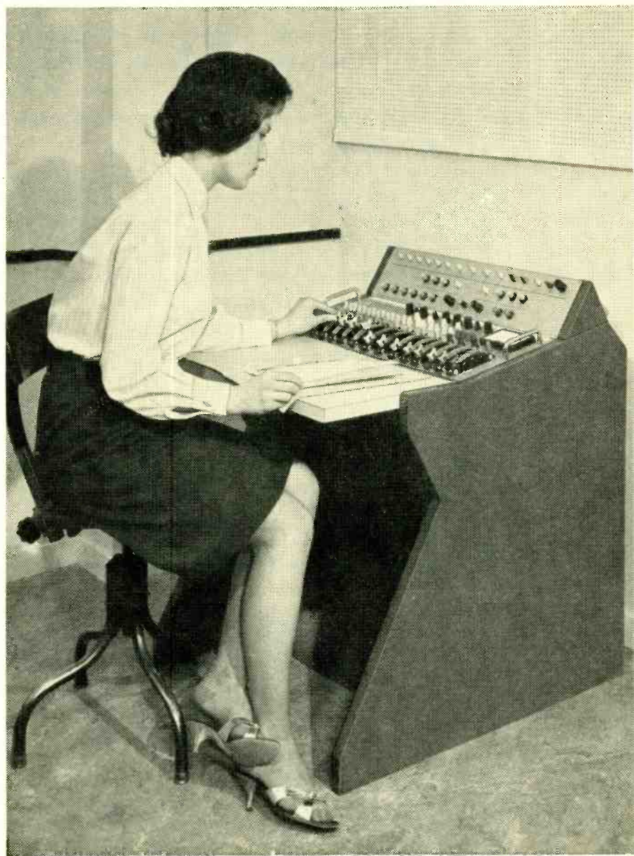
Fig. 4. The basic panel with ancillary echo unit in a typical desk.
