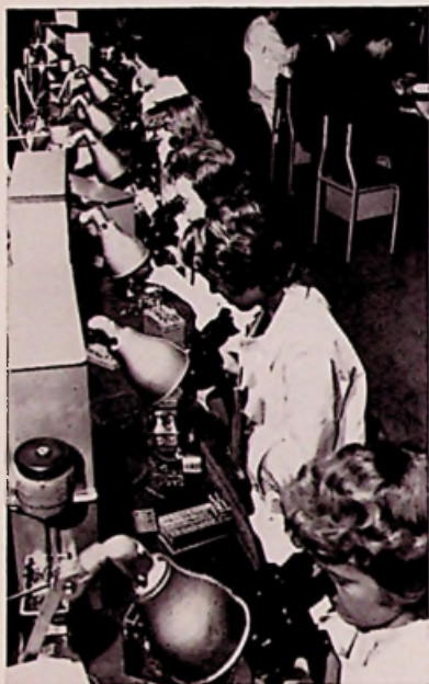
Attaching connecting leads to the emitter and collector pellets. Microscopes are necessary because of the extremely small size of the components.
