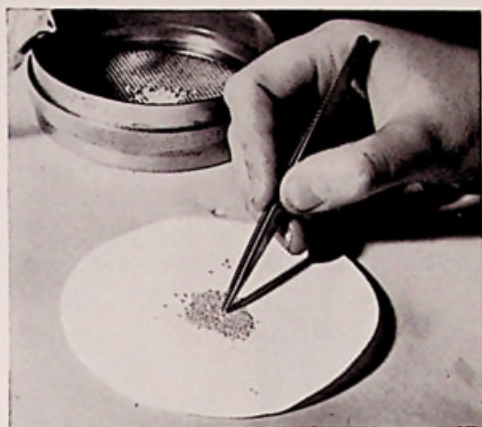
Sorting and inspecting indium pellets for the emitters and collectors
