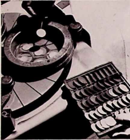
Removing slices of germanium crystal after lapping
