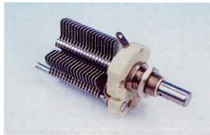
Air dielectric trimmer, SLC Low characteristics. Air gap 0.4mm, 750V tested, air gap 1.15mm 1250V DC tested. Front plate 23.8 x 31.75mm. Values available: 10pF, 15pF, 25pF, 50pF, 100pF and 150pF.
