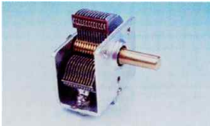
Length (excluding spindle) 23.8mm. AM capacity 10 to 365pF. Tested up to 750V.
