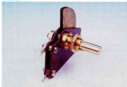
Solid dielectric. Front area 44.5 x 46mm. The following values are available: 6.5 to 300pF, 7 to 500pF.
