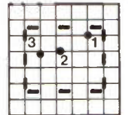
0.1 inch matrix Holes Ø 1.2mm
