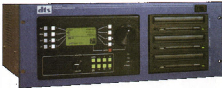
The DTS 6AD digital surround decoder for cinemas. Here, the movie soundtrack is stored on CD-ROMs, and synchronised with a timecode track found on the film. The prototype digital systems must have similar synchronisation arrangements, because the audio and video streams are stored on separate hard disk arrays
