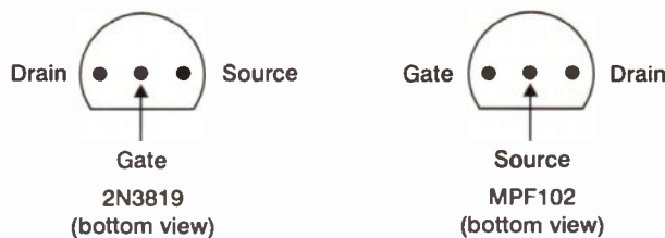
Figure 1. Outline and connections of the 2N3819 and MPF102 JFETs.
