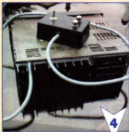
Rear view of the modified Kenwood head unit. The unusual cable exit point on the back of the device is deliberate - this unit is 'removable'. This is one of the reasons for specifying the in-line DIN connections that can be seen to the left of the picture.
