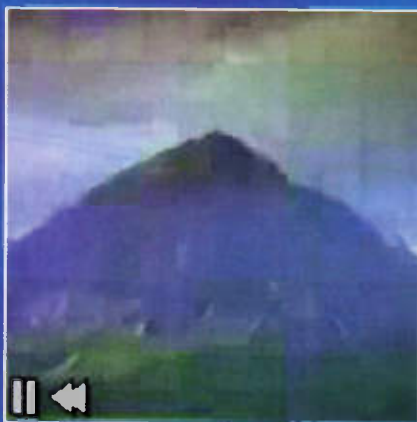
This picture gives you some idea of the best video quality you can expect from the Videophone. Here, the SCT codec has been optimised for 28800bps transfer rates.
