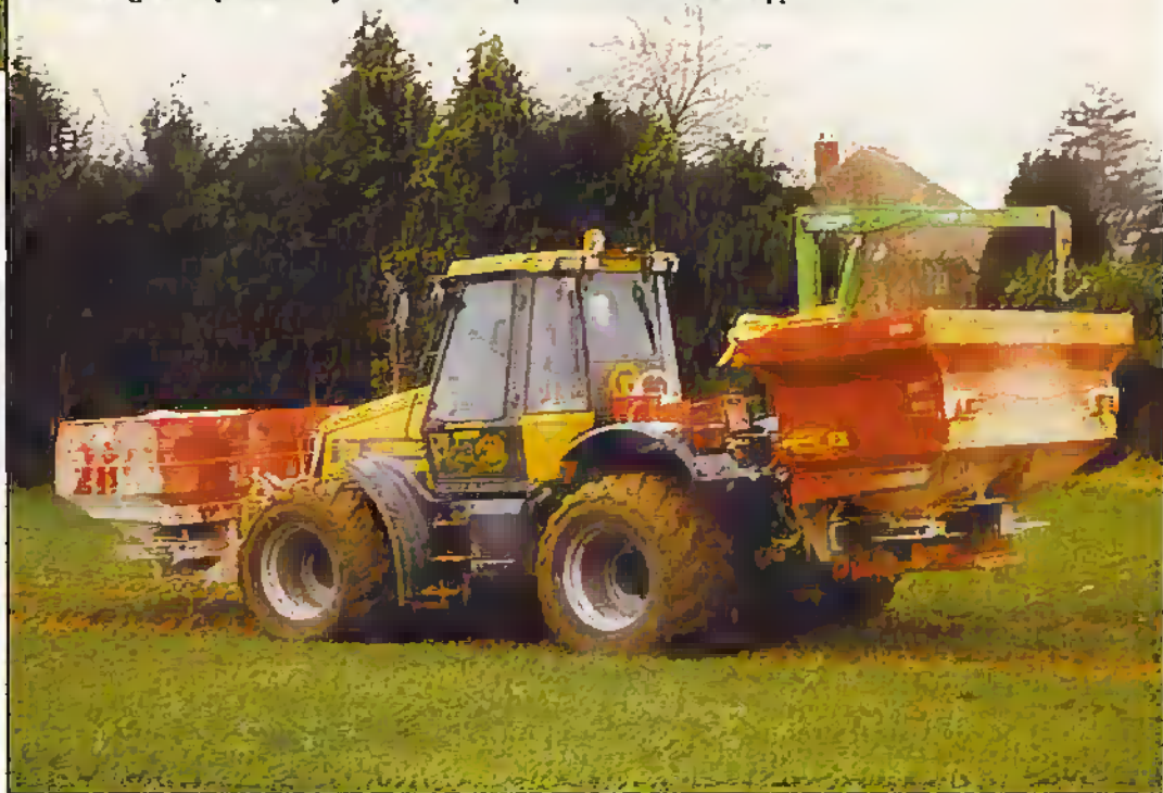
Photo 4b. Showing a pair of fertilizer hoppers mounted on a high tractor fitted with low ground pressure tyres. Note the spinners under each hopper.
