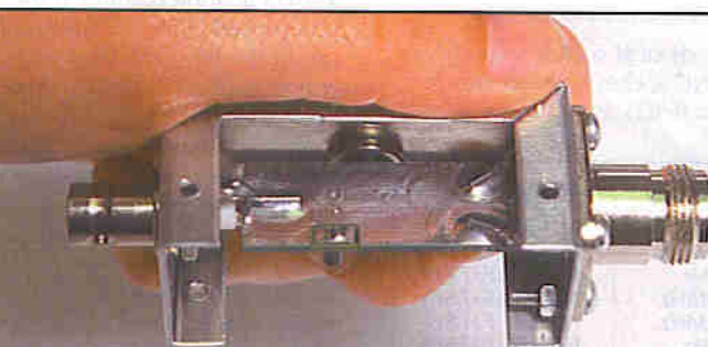
Photo 7e. Completed PSU Interface PCB mounted in the box.
