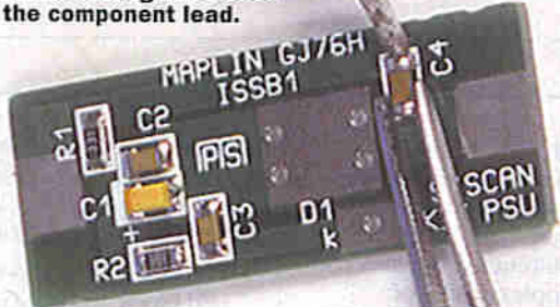
Photo 7b. Reflowing the solder to wet the component lead.
