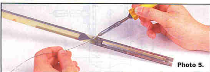
Photo 3 to 6. Assembly of the Aerial PCB. Note use of a low power soldering iron when soldering in the MAR-6 chip.
