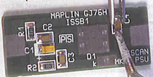
Photo 7c. Making the opposite joint of the component.
