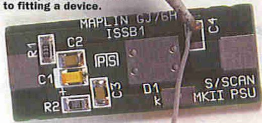
Photo 7a. Wetting the SMD component pads with solder prior to fitting a device.
