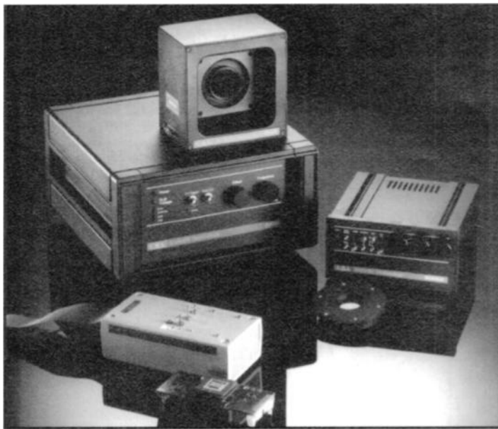
Left: Photo 5. Family shot of CRL Spatial Light Modulators with associated drive circuitry, 2DX320 (upper left); Bistable Optically Addressed SLM (right); SBS 256 (lower left). The Silicon Backplane device is, therefore, significantly more compact than the other devices. (Courtesy of CRL Smectic Technology Ltd.)
