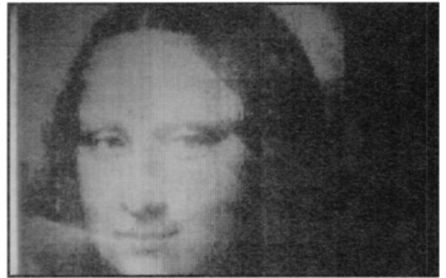
Below: Photo 6. View of a familiar face, to indicate grey scale tones with the SBS 256 silicon backplane device. (Courtesy of University of Edinburgh)
