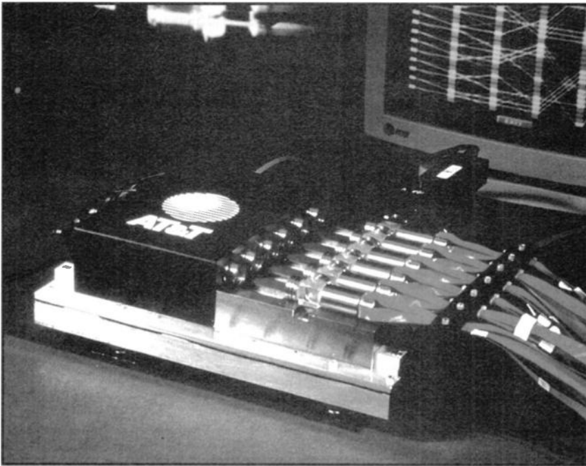
Photo 3. Component of an experimental photonic switching system developed by AT&T Bell Laboratories, which handles 2,048 parallel channels of information. All data in and out is communicated by light beams, and internally more than 60,000 light beams replicate the switching functions. (Courtesy of AT&T Bell Laboratories.)
