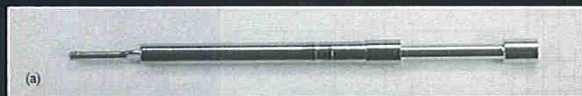
Below: Typical spring contact probes (CSP): (a) Concave type (UL99H). (b) Convex type (UM00A).
