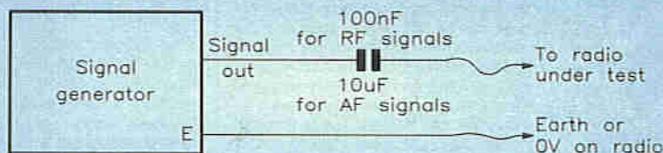
Figure 9. AC coupling a signal generator.
