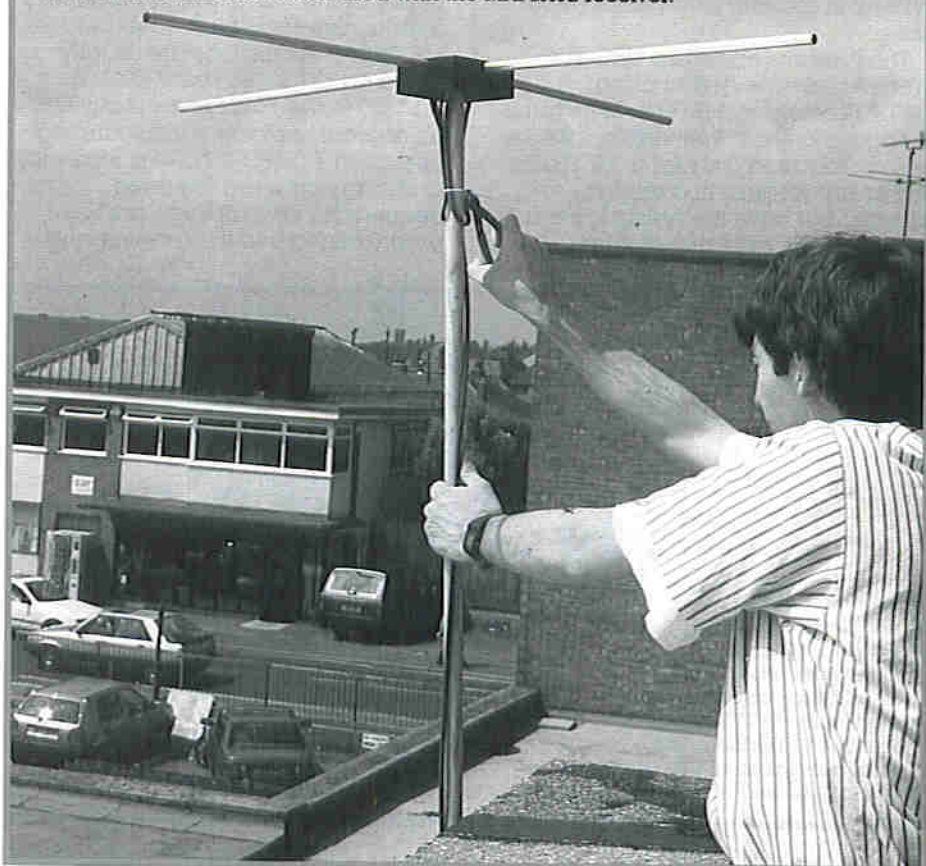
The VHF Satellite Aerial, used for receiving NOAA and METEOR pictures. Simple construction techniques together with highly effective reception, make this aerial ideal when used with the MAPSAT2 receiver.
