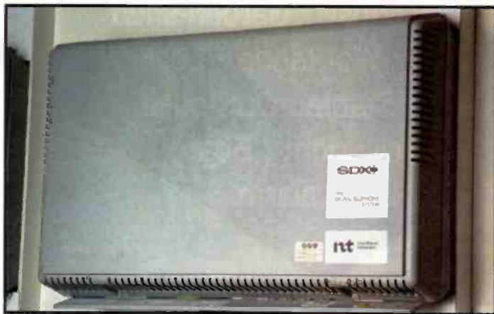
Above left: Photo 3. An ISDN-2 line terminating unit (BT). Above right: Photo 4. A handset enables voice communication on the ISDN-2 line. Below left: Photo 5. An SDX 420N digital exchange unit. Bottom left: Photo 6. Inside the SDX 420N; the ISDN-30 interface card is easily identified by the two white coax cables. Below right: Photo 7. A BT ISDN-30 interface unit; the ISDN-30 fibre optic lines terminate at this unit, with the link to the digital exchange being made by coax cable.
