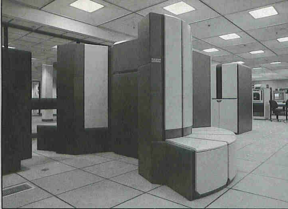
Left: Complex models require complex modelling tools. Shown is the Cray Y-MP8/864 supercomputer (one of the most powerful in the world) at NCAR. It has 64 million words of memory, eight processors (for parallel processing) and can execute an instruction every six nanoseconds.
