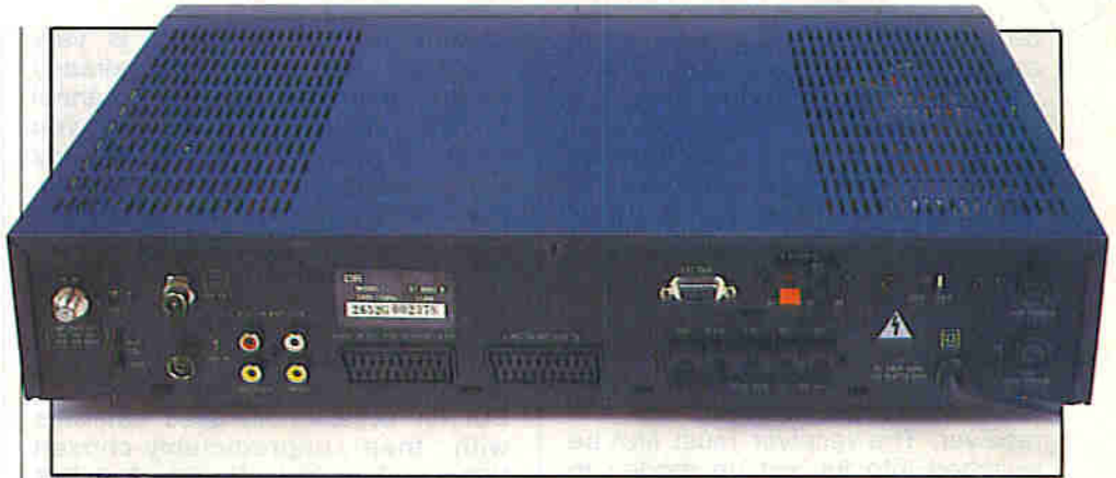
The ST-6002S rear panel. Alas, it loses the 70MHz loop and mechanical polariser connections of its predecessor, the ST-6000S.
