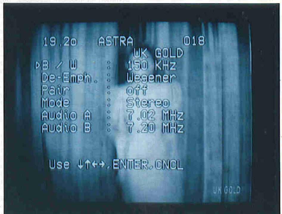
One of the ST-6002's barrage of on-screen menus. This one controls audio parameters (note that one of the audio subcarriers has been deliberately mistuned very slightly – see text). Screen image © UK Gold 1993.
