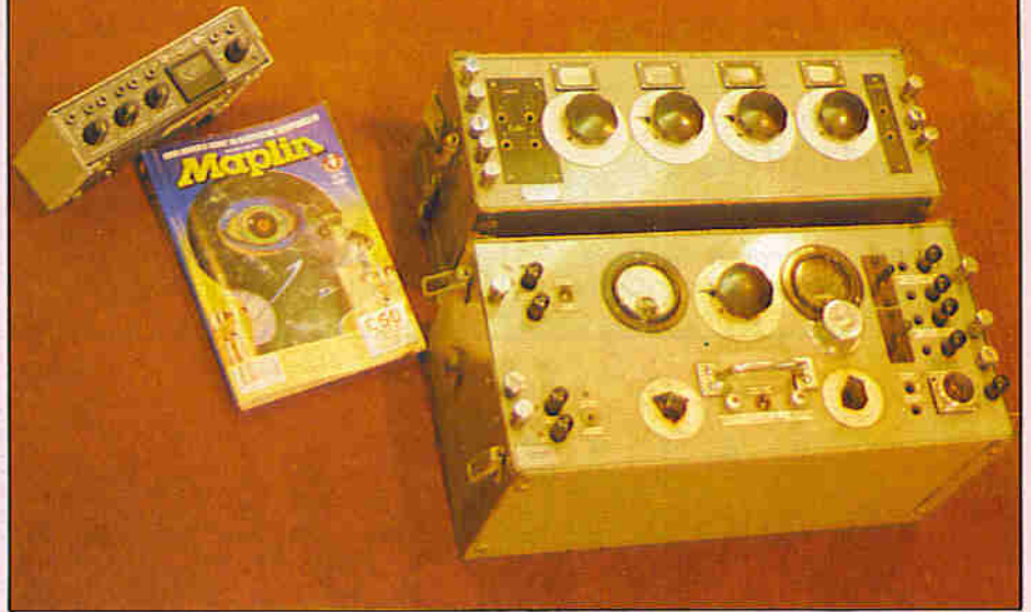
Photo 1. A BBC MX18 portable mixer (top right) with modern equivalent at top left, and OBA8 amplifier (bottom right).
