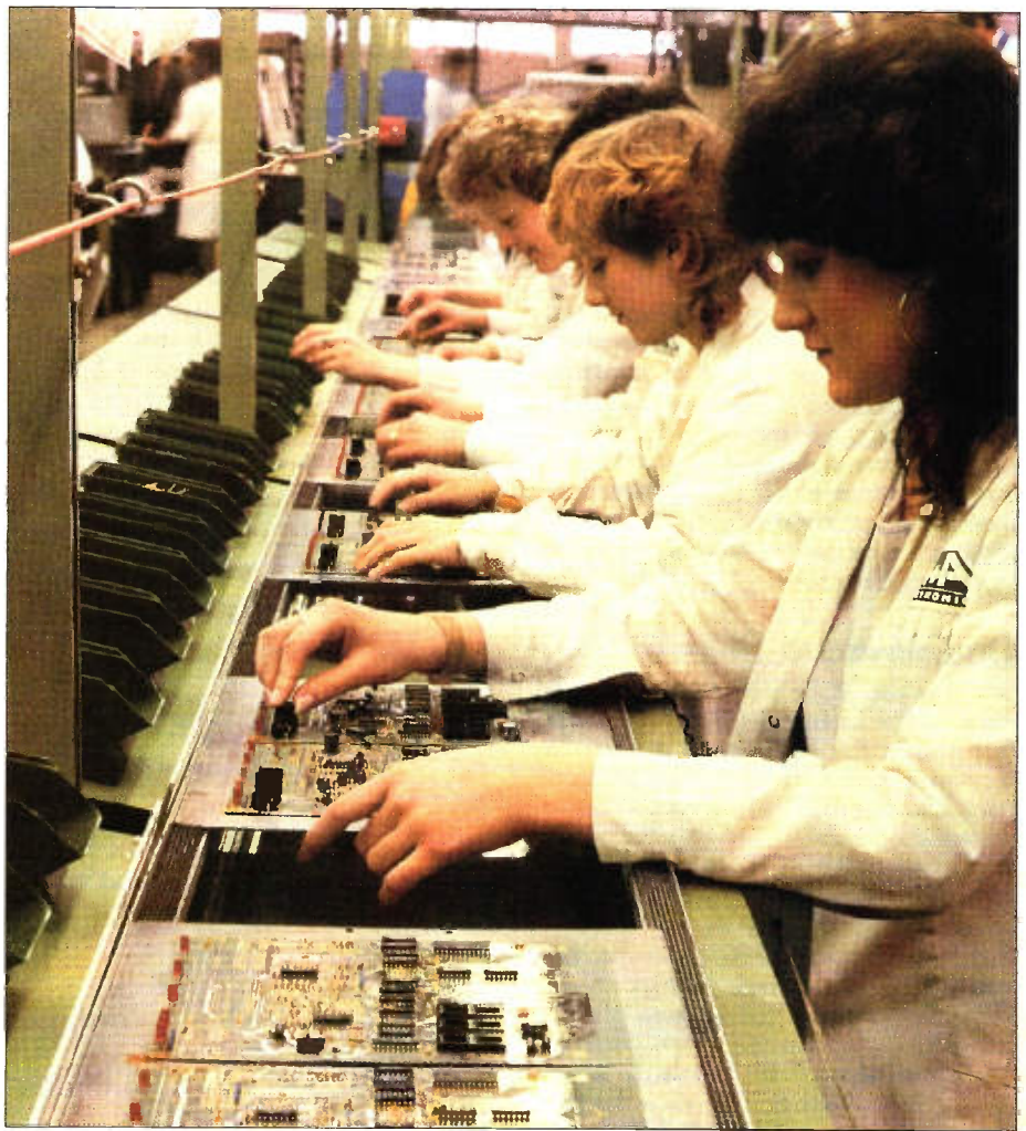
Assembly line, showing operators inserting leaded components into PCB assemblies (PAF).
