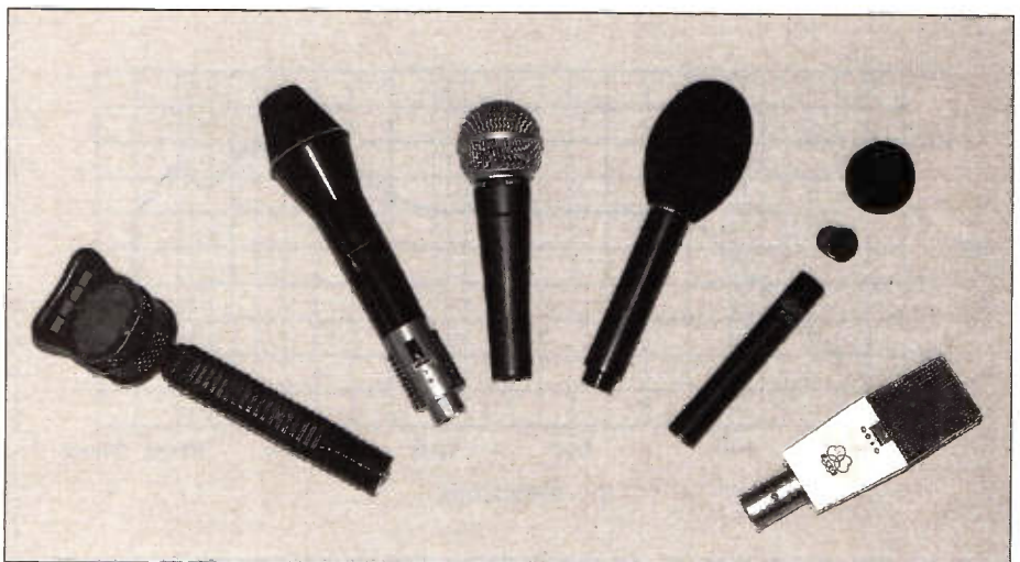
A range of professional microphones – from left to right; Coles Lip Ribbon, AKG D202, Shure SM58, Beyér M201, AKG C451, AKG C414.
