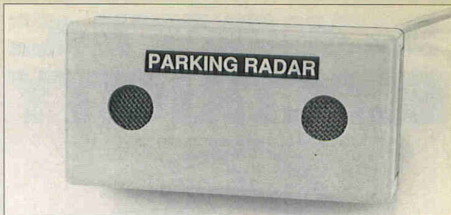
The completed Receiver Unit with protective gauze.
