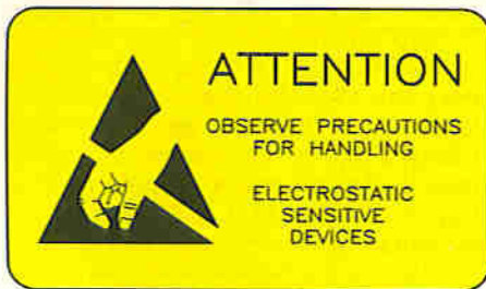
Figure 6. Warning label for electrostatic-sensitive devices.
