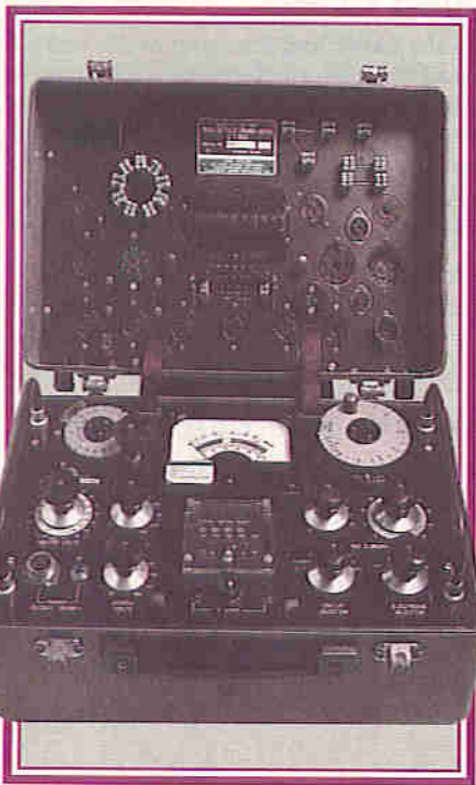
A versatile valve tester, the 'Test Set, Electronic Valve CT-160', produced by AVO for the Ministry of Defence, and now widely available on the surplus market.
