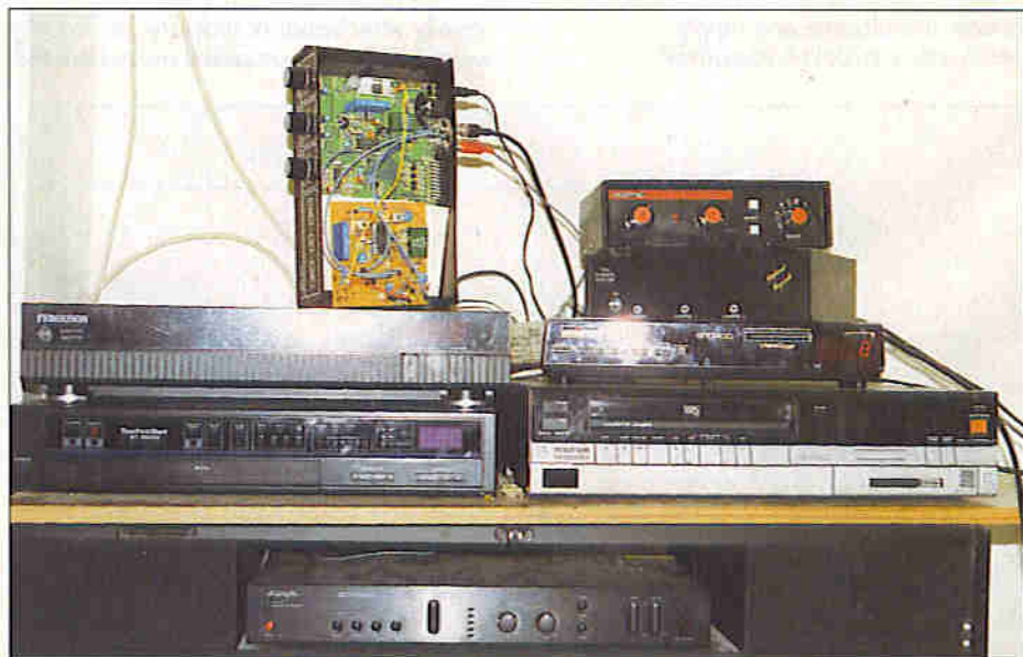
Any more decoding standards to contend with and the shelf may well collapse! On top of the multi-satellite receiver (on the left) are an experimental SECAM transcoder, and a Ferguson BSB receiver fitted with a D2MAC upgrade supplied by Middlesbrough-based TRAC Satellite Systems. On top of the video recorder (going up) are an Amstrad SRD400 (for Videocrypted channels), a now-defunct Filmnet/RTL-4 decoder and an early 'Digisync' sync inserter.
