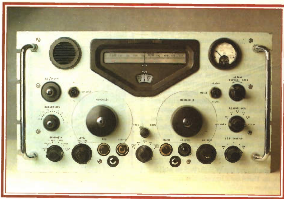
The Racal RA17, a 23-valve communications receiver, covering the range 1 to 30MHz, extending down to 500kHz with slightly degraded performance. The left-hand tuning knob selects the frequency range, while the right-hand one gives continuous tuning over that range. Read-out is on a film scale with an effective total length of approx. 145 feet.
