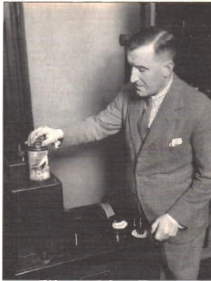
This 1935 photograph, shows the drum, containing the original picture, being loaded into the sending machine.
