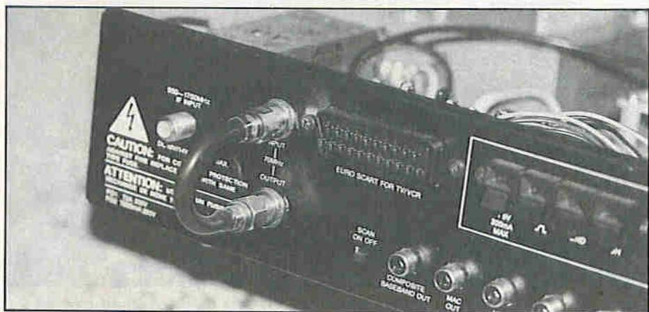
If you use a small dish, reducing the IF bandwidth may help to make the weaker signals watchable. Pictured is a 70MHz loop – now a fading sight from (even the best of) modern multi-satellite receivers – which enables filter networks to be attached.
