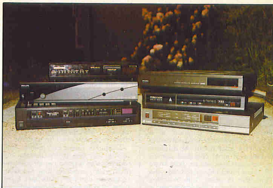
A selection of satellite receivers. Top to bottom, left: Amstrad SRD400 – the first receiver to integrate a Videocrypt decoder; Philips STU-902 BSB receiver – an eventual collectors item; Technisat ST-6000S multi-satellite receiver with 99 channel/30 satellite memory, on-screen graphics and stereo sound. Top to bottom, right: Salora 5902, a highly-regarded 48-channel stereo receiver intended for use with Astra but capable of much more; Ferguson SRA1-S (manufactured, in fact, by Pace) stereo Astra receiver with only 32 channels; Multipoint M1700, an early (circa 1985) 24-channel receiver dating back to the days when you needed a dish of at least 1.5m diameter to receive anything at all.
