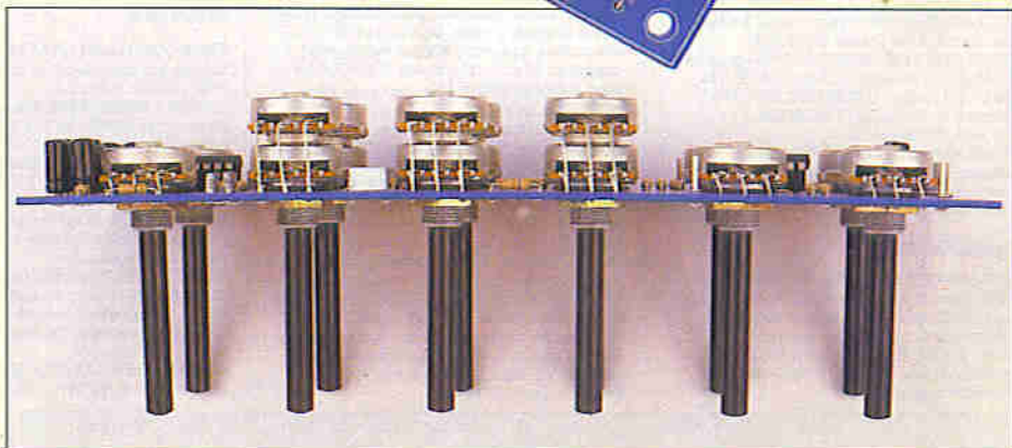
Below: Side view of the Dual Tone Control, showing arrangement of potentiometers.
