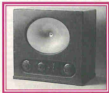
Above left The Brownie Wireless Company's 'Two-Valve Receiver' of 1926. In its moulded black Bakelite case, it was one of the last sets to have externally-mounted valves.
