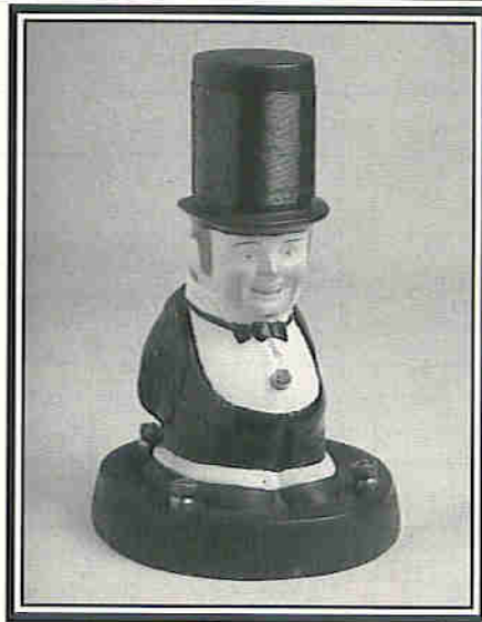
The 'Uncle Tom' Grafton china crystal set. The top hat carries the coil, with a slider at the back for tuning. The crystal is in the form of a diamond shirt-stud, with the cat's whisker protruding from the bow tie. This novelty set, produced in 1924, stands almost 9 inches high.
