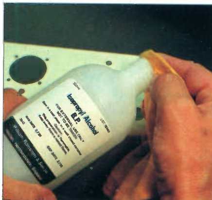
Photo 2. After rubbing down the paintwork, any remaining dust and grease can be removed using some isopropyl alcohol. This can be obtained, in small quantities, from your local chemist.
