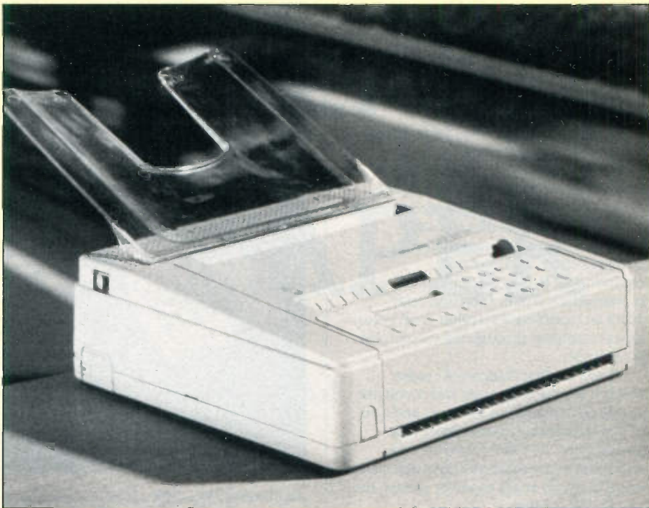
Pitney Bowes' 9000 model can transmit and receive in as little as 6.3 seconds, utilising new standards in error correction.
