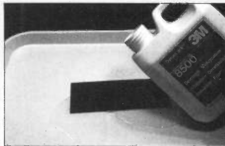
Photo 7f. Having exposed the label, place it in a plastic dish and pour a small amount of 3M developer over its surface.
