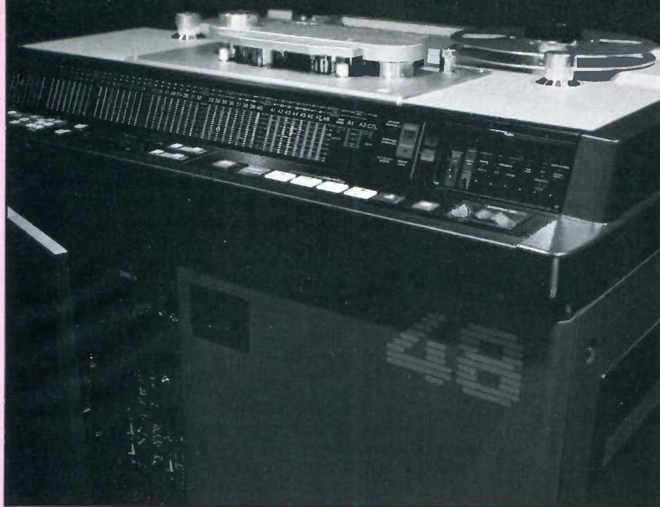
A tape recorder and a half – 48 digital tracks on the Sony PCM 3348 in Studio 2.
