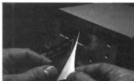
Photo 7h. After rinsing the label under running water, dry and remove the paper backing. Carefully place the label onto the metalwork of your case.
