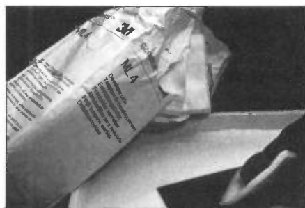
Photo 7g. Using an ML4 pad, begin development by using light figure-of-8 movements to remove most of the background coating.
