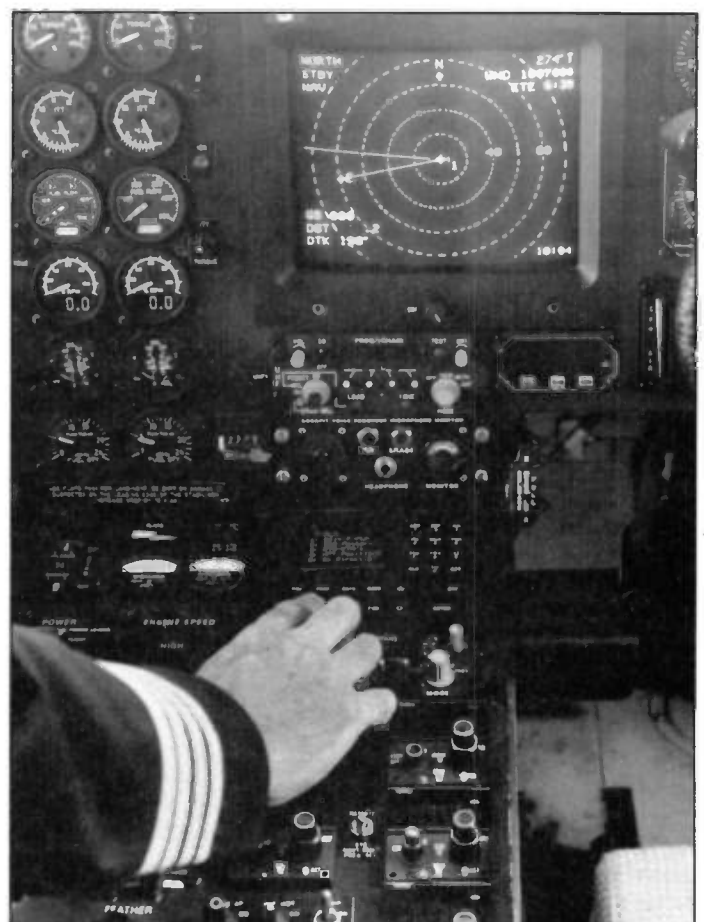
Racal Avionics RNS 5000 worldwide navigation management system – Above left: Installed in an Embraer Brasilia aircraft. Above right: Installed in a major civil aircraft.
