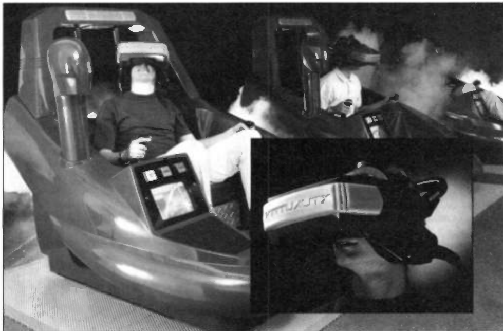
The arcade 'sit-down modules'. Inset: The 'Vissette' visor generates an internal 3D display on LCD screens.
