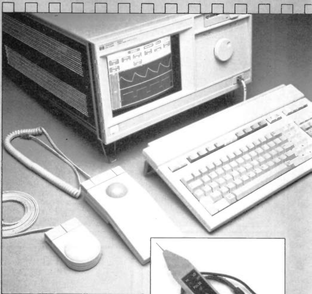
Top: The Hewlett-Packard HP16500A Logic Analyser System – an example of the current state-of-the-art. This unit can analyse up to 204 data channels, each with a data rate of up to 50 million bits per second. A colour touch-screen with pop-up menus ensures ease and quickness of set-up and use.
