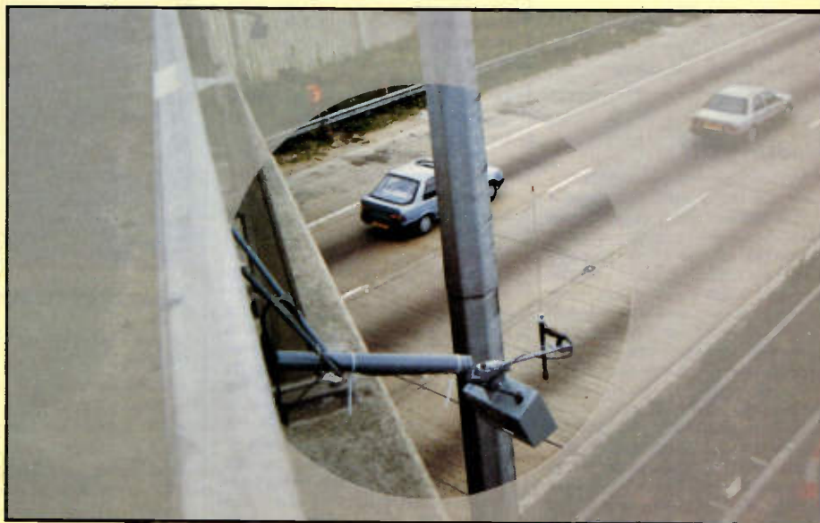
Photo 1. Infra-red sensors in use on the motorway network.
