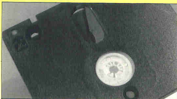
Photo 2. The shutter of the 3in. disk has been partially operated to show the disk access slot partly open; the actual disk surface is clearly seen. At the bottom is the index hole, just opening. The small hole (arrowed) top left is the write protect hole.
