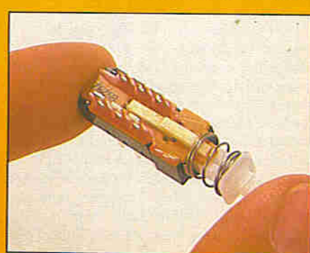
Photo 3. Switch ready for mounting on 6 way bracket.
