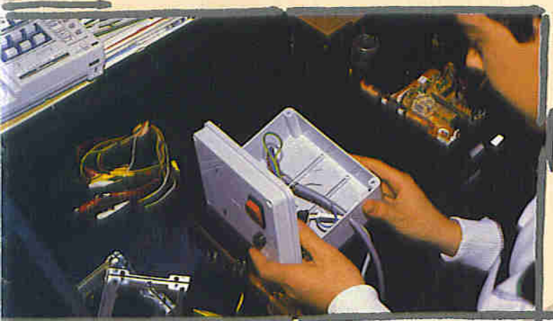
The mains isolation unit under construction.
