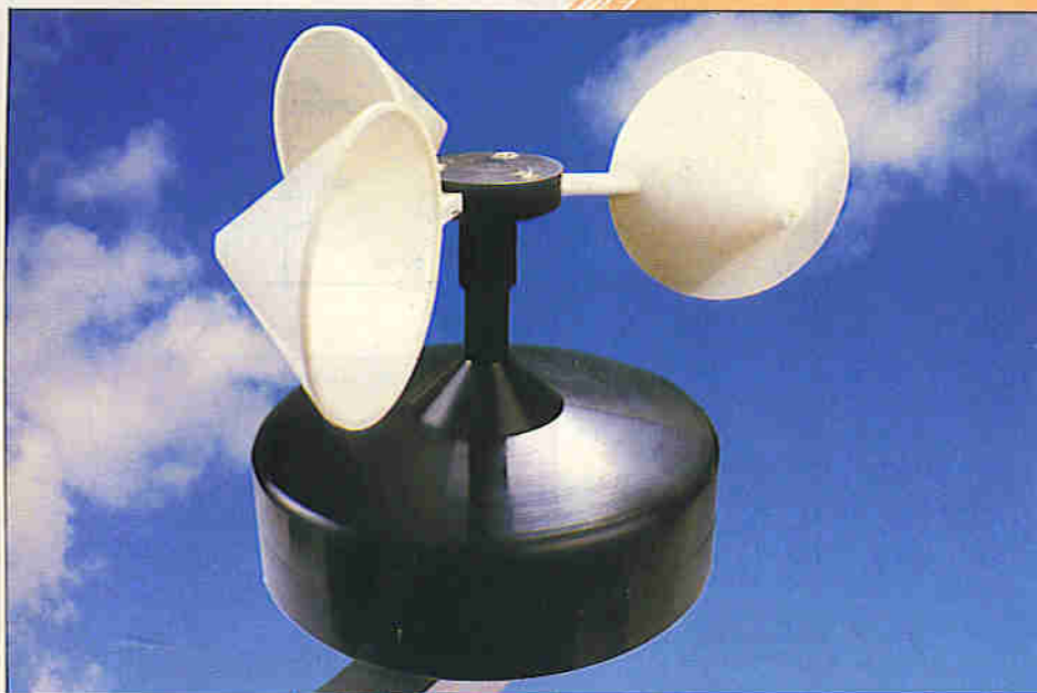
Photo 1. The wind speed cups.
