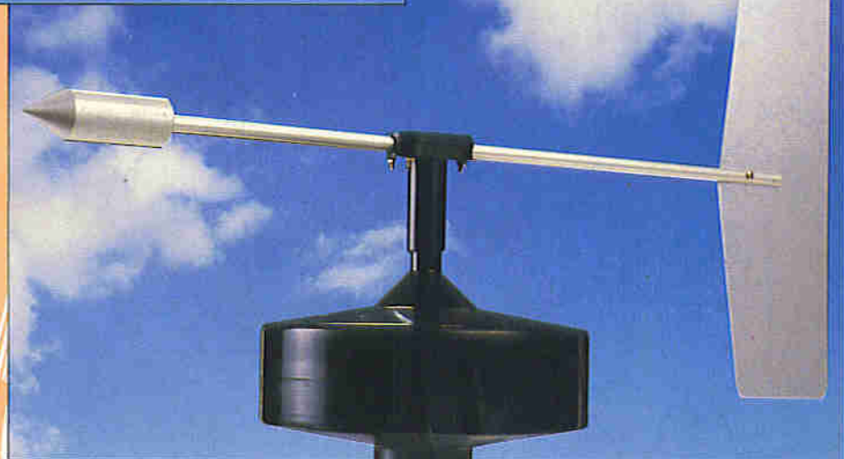
Photo 2. The wind direction 'arrow'.
