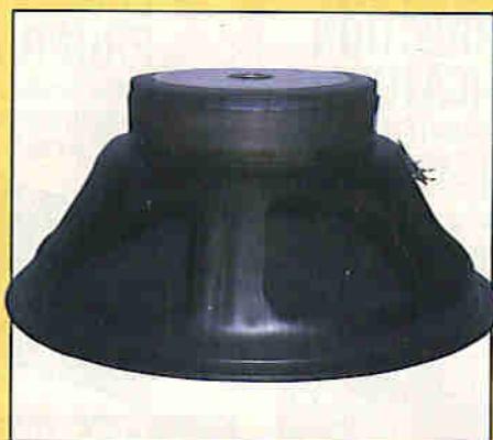
Photo 1. Goodmans Audiom 12P-D, a typical 300mm bass driver for sound reinforcement or electronic music.
