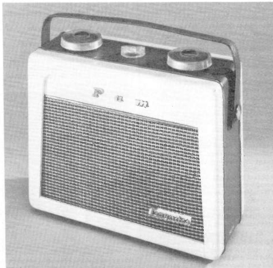
The first transistor receiver in production in the UK, the PAM 710 of 1956.
