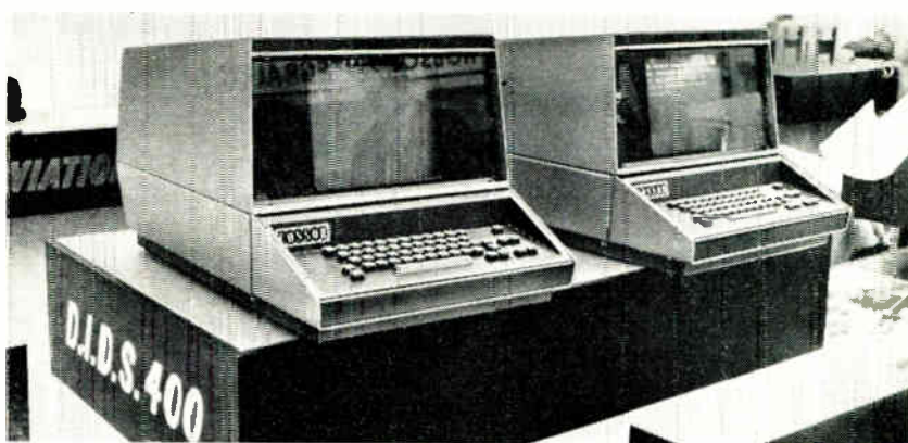
▲ Cossor were exhibiting their digital information display system, DIDS/400. This can be linked to a computer to provide a display of information such as aircraft seating plans, passenger lists or any other required data. Clear characters and symbols are provided on the c.r.t. display and a keyboard facilitates the input or editing of data (79)
