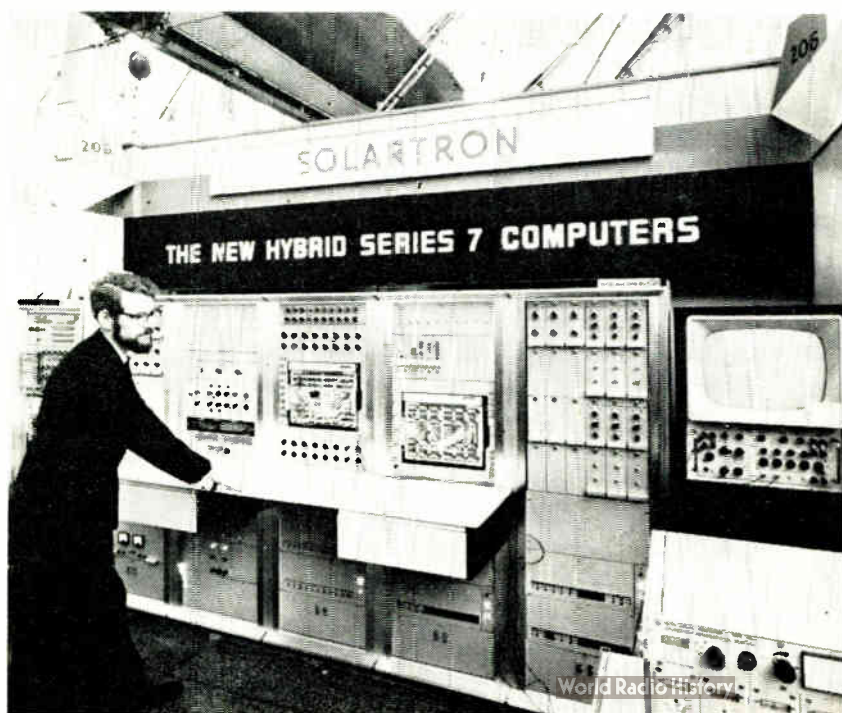
▼ This computer is one in the Hybrid Series 7 computers exhibited by Solartron. These analogue machines will function with digital computers to provide a system offering both digital and analogue techniques. Patchboard programming is featured and an error indication and fault-finding facility is included in this and other computers in the range (81)
