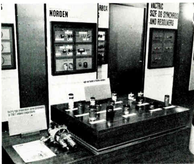
This shows the display of Norden encoders exhibited on the Vactric Control Equipment stand. Various types of encoders and analogue-to-digital converters are available including both brush and magnetic types. Units for various binary codes can be obtained (88)
