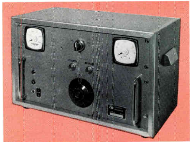
Here a standard tachometer can be seen installed on the left-hand side of this speed and acceleration control unit
