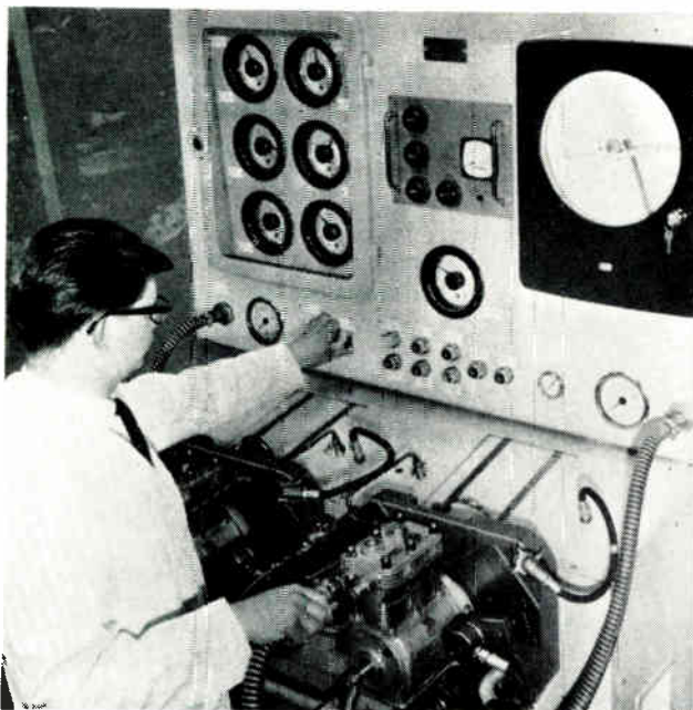
This programmed test rig is constructed of standard equipment such as the tachometer illustrated on the next page
