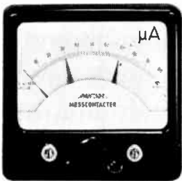
Left: PANTAM pointer indicator with photoelectric contacts. Right: PANTATHERM electronic temperature controller.
