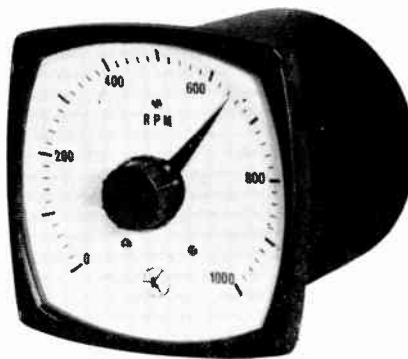
Fig. 6. The solid-state calibrated control instrument used to control the speed of a 10 h.p. commutator motor
