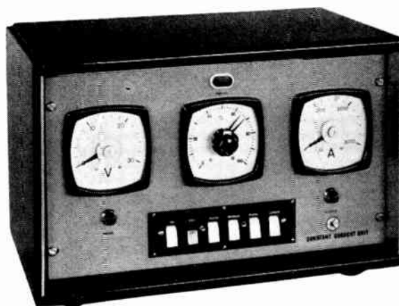
Fig. 8. A solid-state calibrated control instrument which incorporates saturable-reactor elements for regulating currents of up to about 5,000 A
