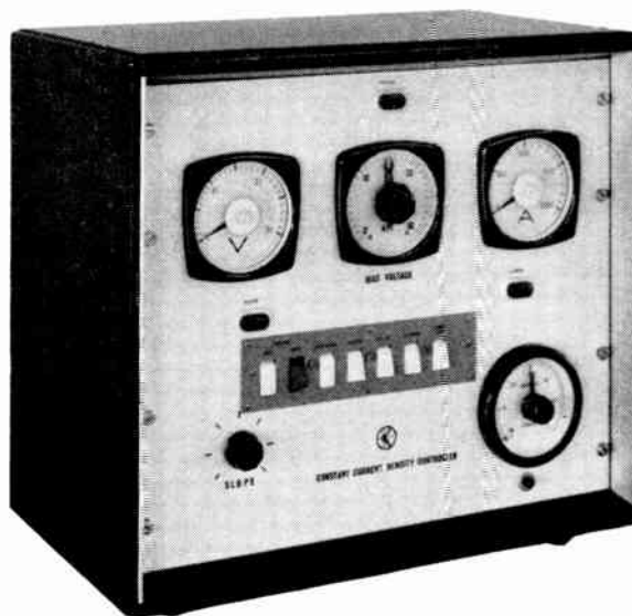
Fig. 7. The control unit of a constant current-density instrument used in electro-plating applications
