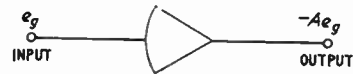
Fig. 1. High-gain amplifier. The input voltage is multiplied by gain A ( 10^8 or greater); minus sign indicates phase reversal in amplifier
