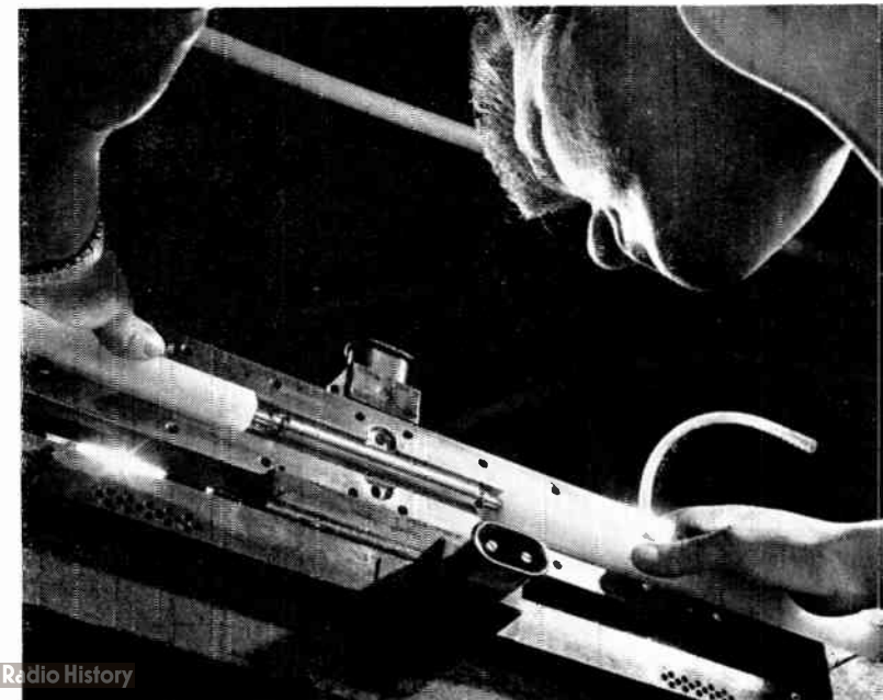
▲ Uninterrupted power for SEACOM is available from the equipment that feeds a closely-controlled direct current through the centre core of the cable (which is also carrying 80 or 160 two-way conversations) to operate the repeater amplifiers along the route. Very close control of current is essential to ensure that the repeater valves are not subjected to any strain that will shorten their 20-year design life. Equipment like this is installed at each shore terminal station and is designed in such a way that failure of one terminal through fault or power interruption will not put the cable out of action
