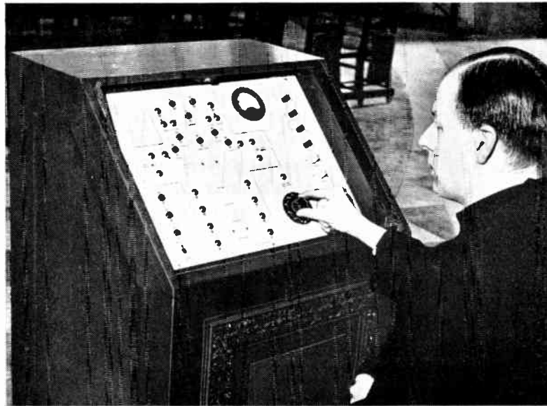
Fig. 8. An operator at the remote control panel. The lamp immediately above the gain control lights if the erase oscillator fails and at the same time the recording system is taken out of operation
