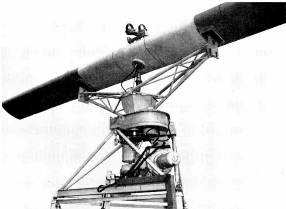
This shows a close-up of the SECAR aerial and turning gear, taken from the rear. Modification kits, including a special rotating waveguide joint, are available to mount the SECAR aerial on any Marconi or CFTH primary radar aerial system
