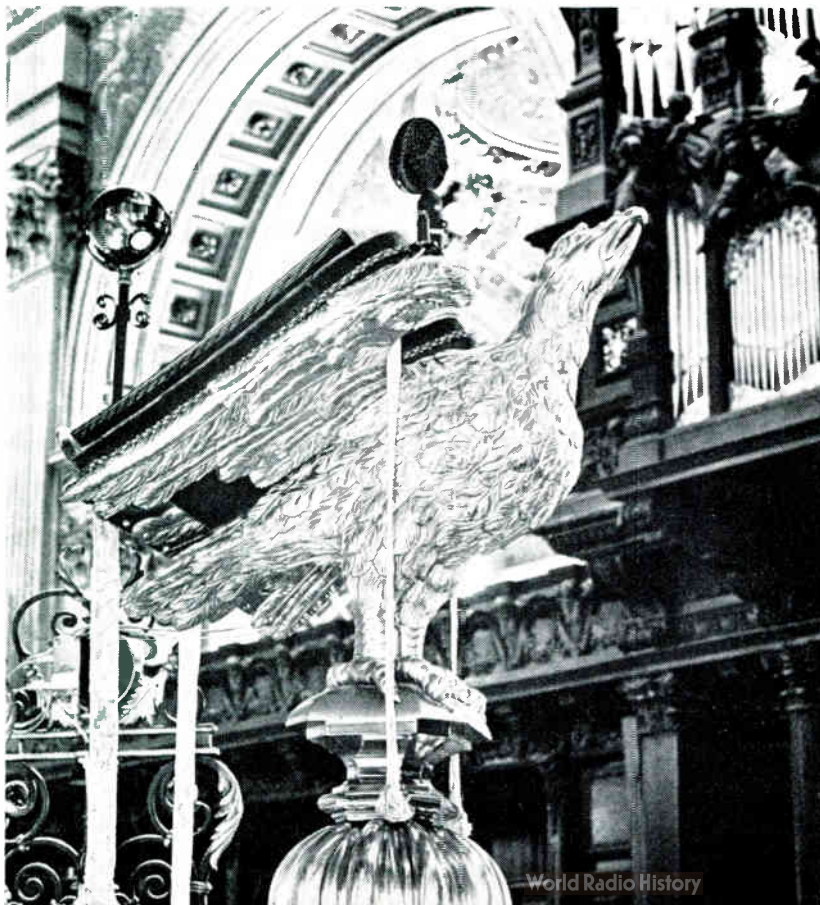
Fig. 4.(a) Typical microphone and mounting shown on the lectern. The small assembly at the side of the microphone carries a signal lamp. (b) The relationship of the directional microphone and loudspeaker at the lectern
