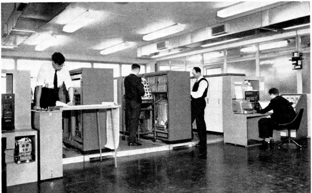
The computer now finds a place in communications networks to control the routing and switching of messages. Standard Telephones and Cables Ltd. have produced the 8300 ADX system for this purpose. At a switching centre the computer examines all incoming messages for destination, priority and security and routes them accordingly.
