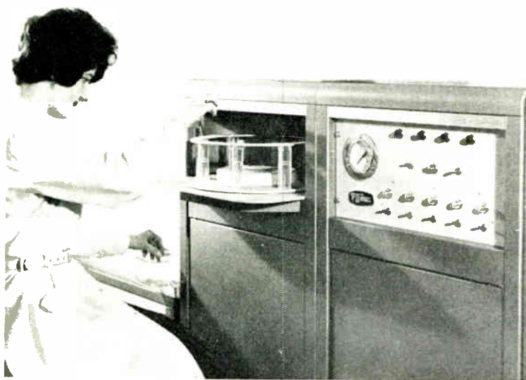
This automated leak detector, demonstrated by 20th Century Electronics, will vacuum test individually up to 1,000 devices per hour. Any that leak are rejected. Maximum dimensions for components are 0.5-in. dia. \times 2.5-in. long. The leak rejection threshold may be set to less than 10^{-5} l/ \mu sec (57)
