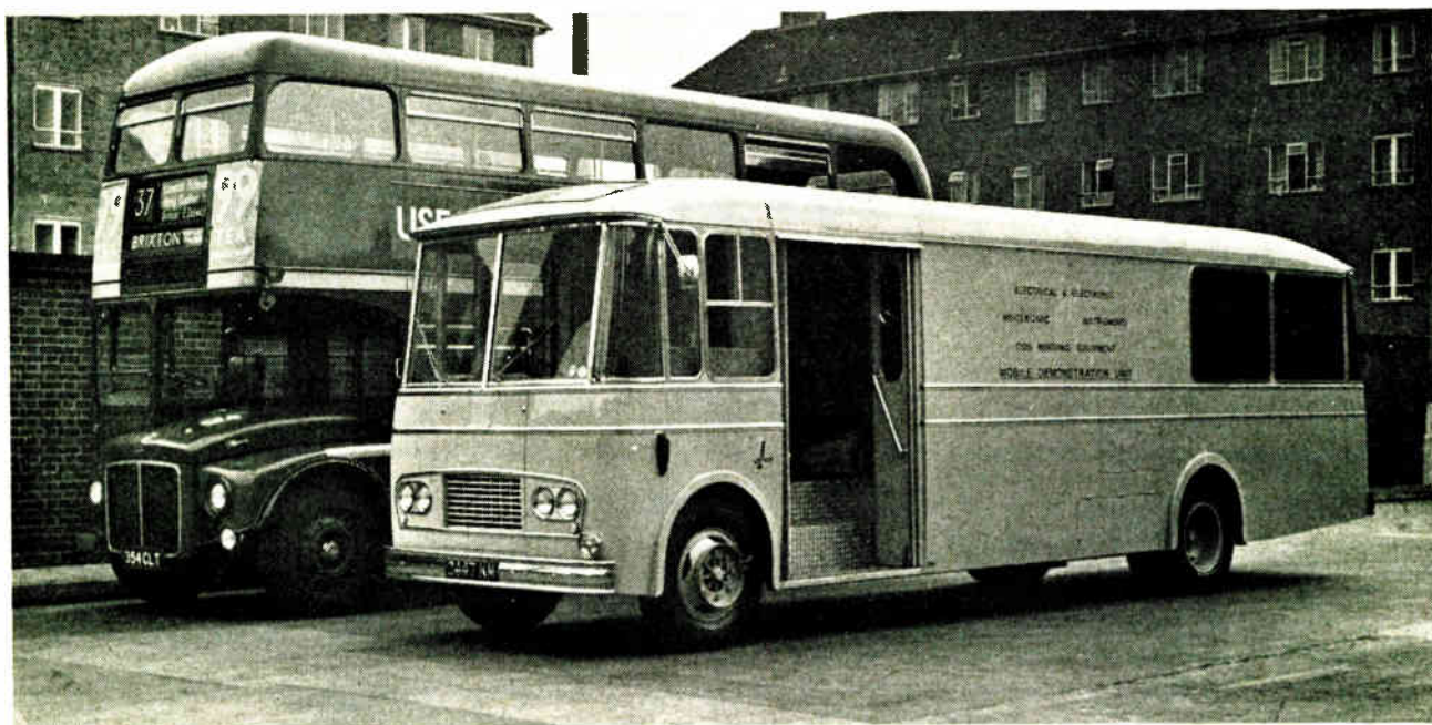
This mobile demonstration unit, shown for comparison alongside a London bus, was recently commissioned by Avo. It has been designed mainly for Continental use and can accommodate a complete range of testing and measuring instruments as well as coil-winding machinery
