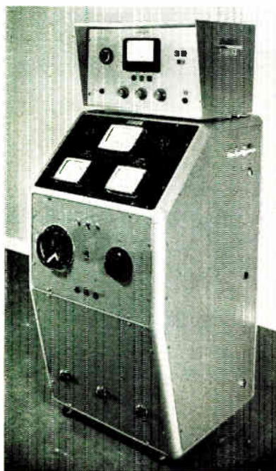
Illustrated here is the G. V. Planer electron beam heating equipment with a controlling ratemeter. This is suitable for the vacuum deposition of metals and non-metals. It is designed for either direct electron beam heating of the evaporant or for indirect heating, by electron bombardment of the evaporant container. The direct heating system produces higher temperatures and hence permits evaporation of more refractory materials (67)
