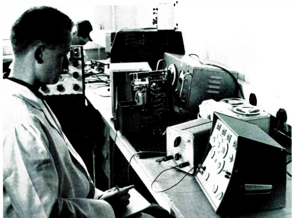
If both amplitude and frequency of a noise vary with time, the noise can be recorded and played back to the statistical analyser through an octave band filter
