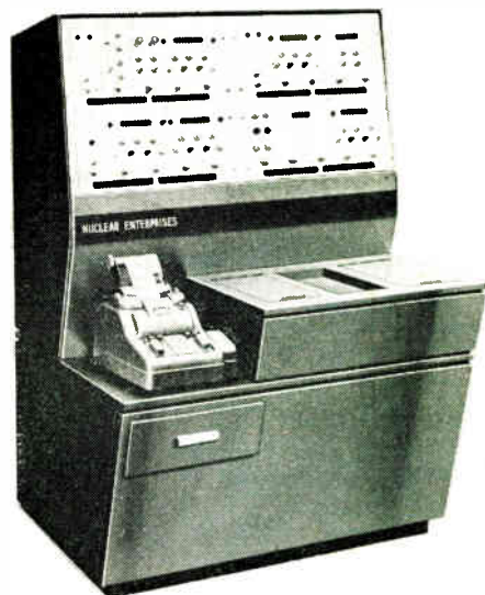
Nuclear Enterprises were showing this dual-channel automatic liquid scintillation spectrometer type NE8303. Designed to give low-cost fully automatic counting, it uses transistor modular construction. Measurements may be made at high efficiencies of tritium, carbon-14, iron-55 and other radiostopes with up to 60 samples being handled in rotation or in selected batches (74)
