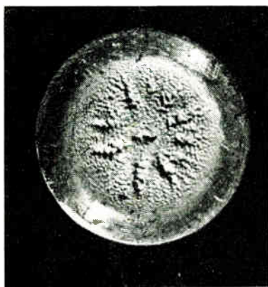
The erosion of the end of a stainless-steel probe of 1/2-in. diameter brought about by 100 hours of cavitation. The scale is of mm
