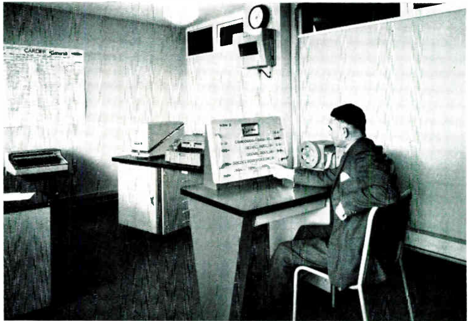
General view of part of Continuous Process Control Unit at Cardiff. Left to right are the keyboard, high speed output punch, typewriter, control panel and low speed output punch of the English Electric KDN2 computer. Under the clock is a digital read-out screen for abstracted data
