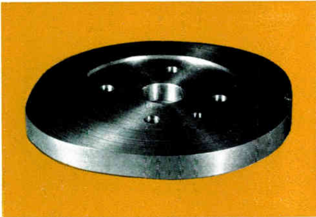
Fig. 8. Cam machined on tape-controlled Newall 1520 machine. Profile surface finish is 6.5 microinches centre-line average
