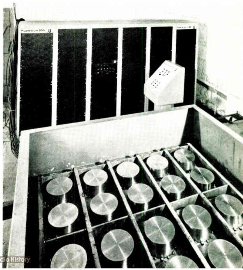
Rapiclean 900 ultrasonic cleaning plant, showing the coupling units
