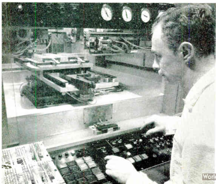
About half the wiring of the Honeywell 400 computer is handled by this automatic wire-wrap machine, which can perform eight complex wiring operations per minute
