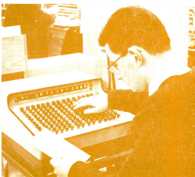
Columns of keys are arranged to allow input of command, train number, location number, wagon type number, state and quantity. This is one of two keyboards used for injecting train composition data which goes to transit store
