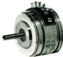
A forerunner of group of special potentiometers based on international (N.A.T.O.) dimensions was featured by Salford Electrical. Known as their frame size 11 unit (approx. 1-in. diam.), it is a 2 W wirewound unit with values from 500 \Omega to 50 k \Omega ( \pm 5\% ). Resolution is from 0.15% to 0.06% and the linearity is \pm 0.5\% . Up to 12 extra taps can be provided and up to 4 units can be ganged together in any phase (51)
