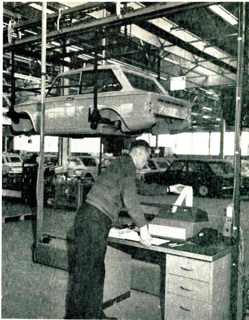
▲ A supervisor taking production data from the output printer at the pre-mount point in the final assembly line
