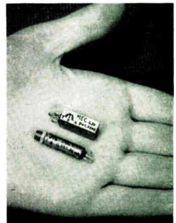
This Ancillary Developments A.D.O. 'Oxipot' trimmer potentiometer indicates a trend in the type of component. It is believed to be the first of its kind to use an oxide film element. It can be produced in values up to 3 M \Omega ( \pm 20\% ) with a power rating of 0.1 W and it maintains its stability over an ambient temperature range of -50^{\circ}\text{C} to 150^{\circ}\text{C} (54)
