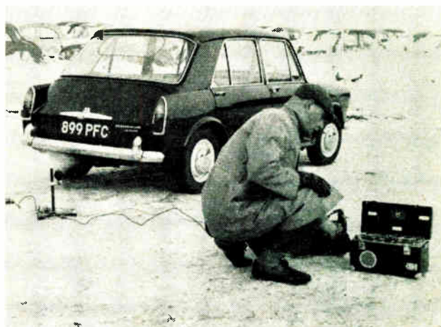
Exhaust noise from a Morris 1100 being recorded
