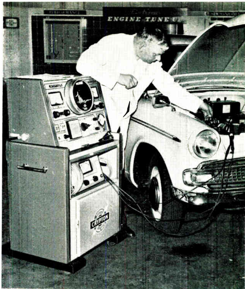
Crypton Motorscope engine tester connected to an engine
