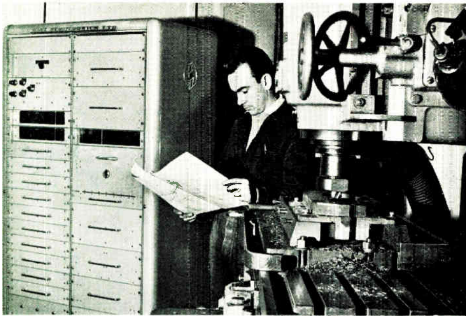
C.I.C. Engineering, manufacturers of shoe moulds, are using a Cincinnati No. 3 milling machine with an E.M.I. Electronics control system. Punched paper tape is used and left and right foot moulds can be cut from the same tape merely by turning a switch
