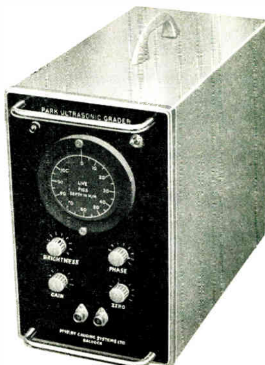
The simple arrangement of controls is clearly shown in this close-up view. The model illustrated has a circular measuring scale instead of the horizontal one described in the text
