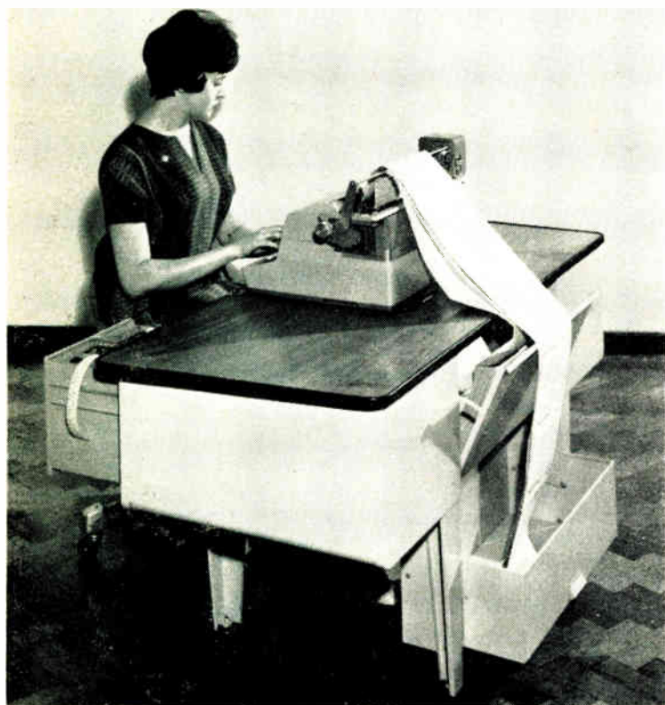
The type 300 Synchrotypewriter perforates seven-channel paper tape as a by-product of invoice typing. By keeping tape units in slide-away drawers and continuous stationery feed and refold at the back of the desk unit, a completely uncluttered work service is provided for the operator
