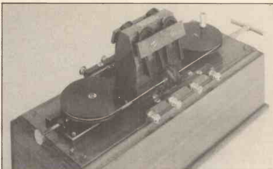
Marconi's Magnetic Detector, from about 1904.
