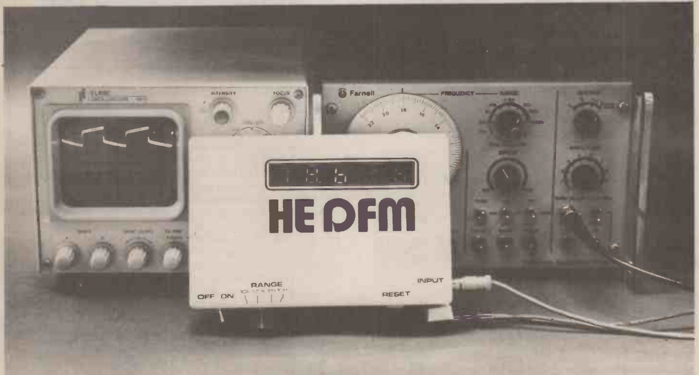
The HE Digital Frequency Meter hooked up to our workshop signal generator and oscilloscope for calibration
