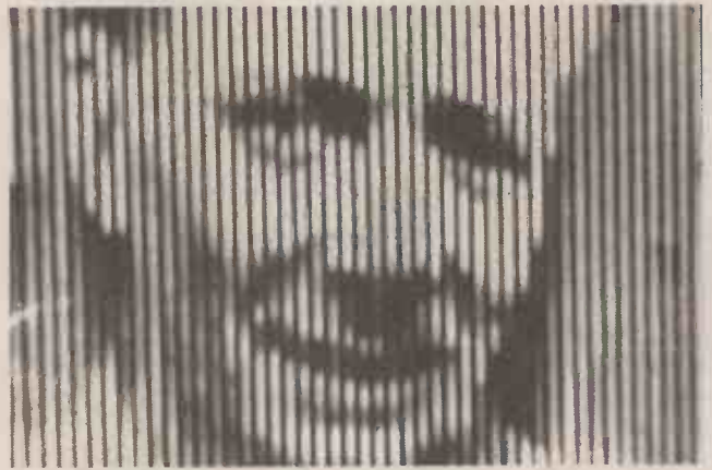
Photograph from a CRT screen of a 48 line picture. Pictures of this quality are easy to duplicate on relatively simple equipment. (The use of a CRT for display is simply to produce a better photograph.)
