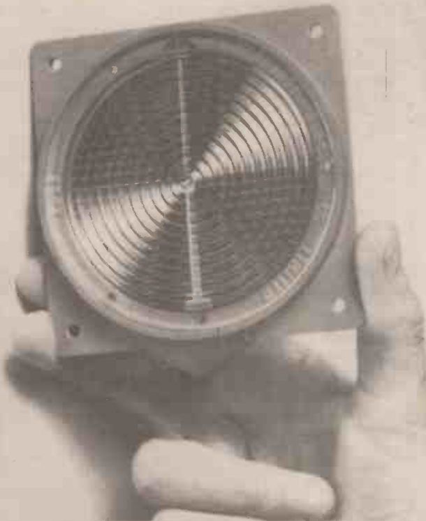
This is the Ferranti ESC-3 Silicon Solar cell module. It is primarily intended for experimental use and will deliver 0.5 V at 0.8 A in bright sunlight
