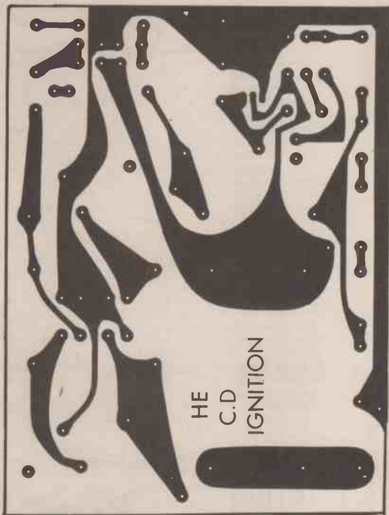
Fig. 2. Above. PCB layout for CD ignition.
