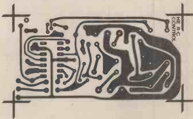
Fig. 2 (left) Overlay diagram for the R/C Motor Speed Controller.
