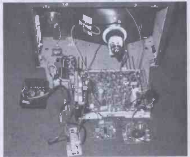
The business end of a TV receiver. This particular model is a particularly good example of state-of-the-art TV technology. It is the Rank Toshiba X53 colour set. In this picture the set has been stripped down to show the various parts of the receiver. Inside the cabinet are the tube and speaker. The main board in the foreground contains all of the electronics for signal demodulation and tube drive, the tuner unit can be seen on the flying lead (far left).
