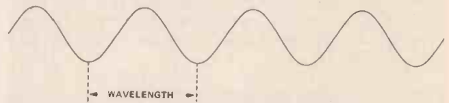
Fig. 1. The wavelength is the distance between neighbouring peaks of the same kind.
