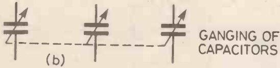
Fig. 7.6b Using ganged capacitors to tune several stages simultaneously.
