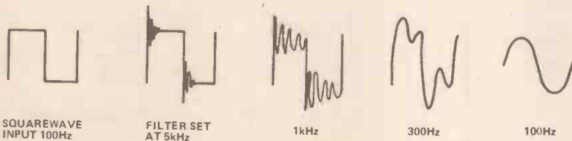
Fig. 7. Using a low pass filter, with a Q of 5 to "ring" the harmonics of a square wave.
