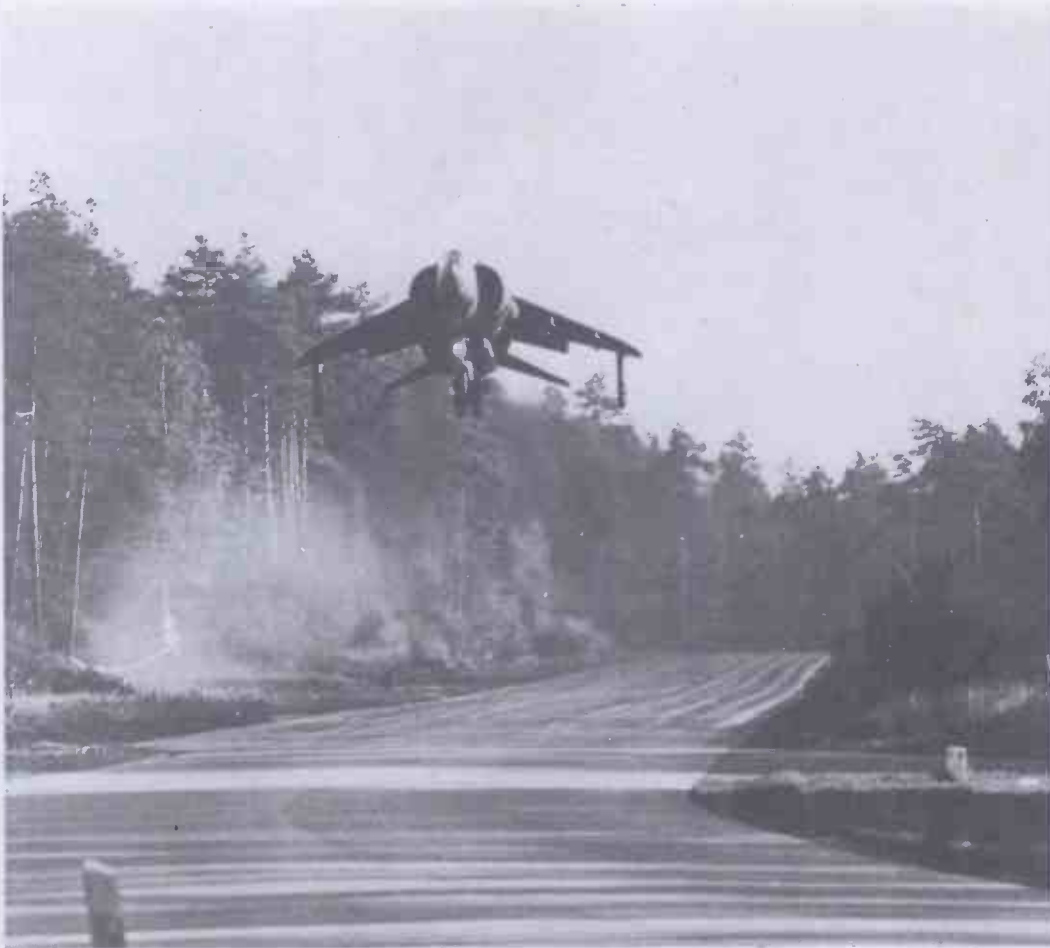
An RAF HARRIER operating from Gutersloh in West Germany. These VTOL (Vertical Take-Off and Landing) fighters can operate from any clearing large enough for them to sit in, and by virtue of their excellent low flying abilities form a powerful (dispersed) strike capability.
