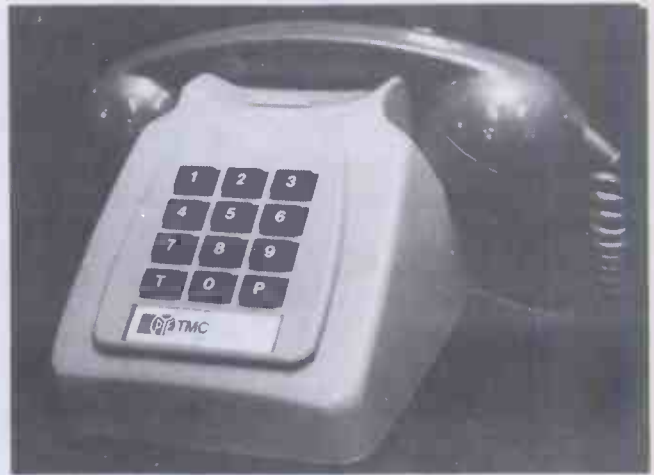
Pye TMC X-Press Callmaker keyphone (£7 a quarter from PO) which stores 10 numbers and allows the last entered to be redialed by pressing a button.
