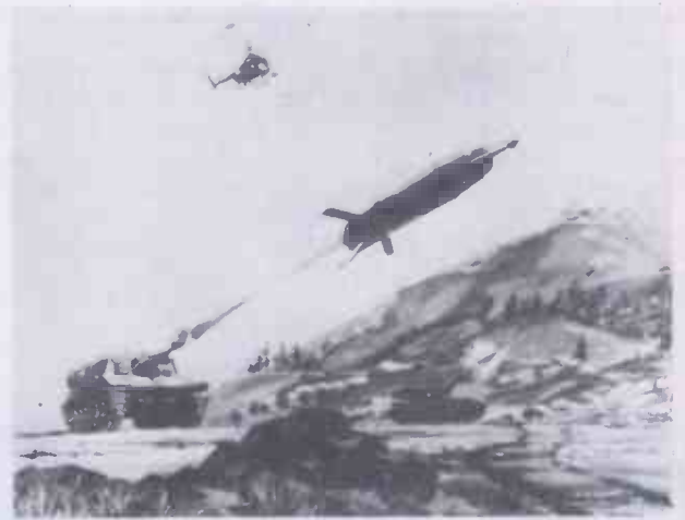
ORLANDO laser-guided projectile being fired from an M109 self-propelled artillery vehicle.
