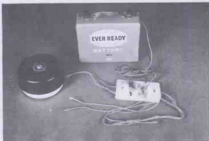
The Cistern Alarm connected to the bell and battery.
