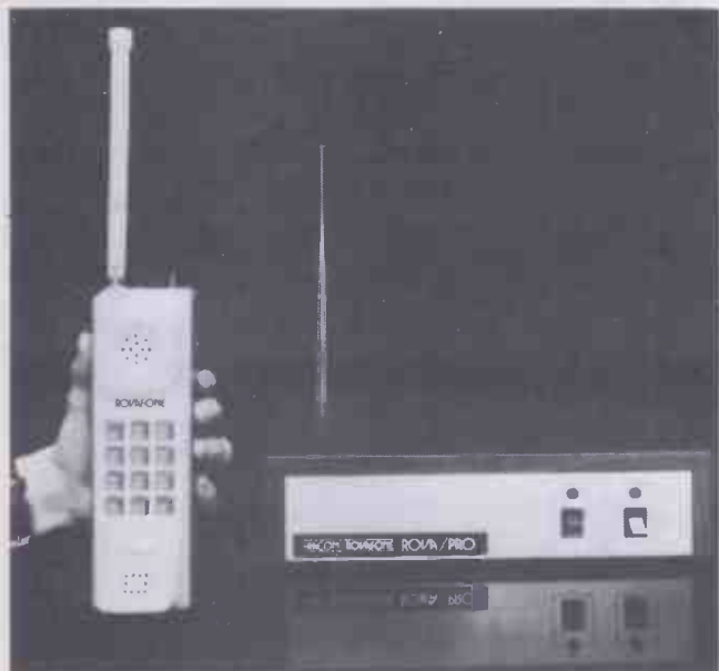
In the United States, CB radio and telephones technology combine to offer fully portable telephones without any wires, but with full outgoing dialling and incoming ringing.
