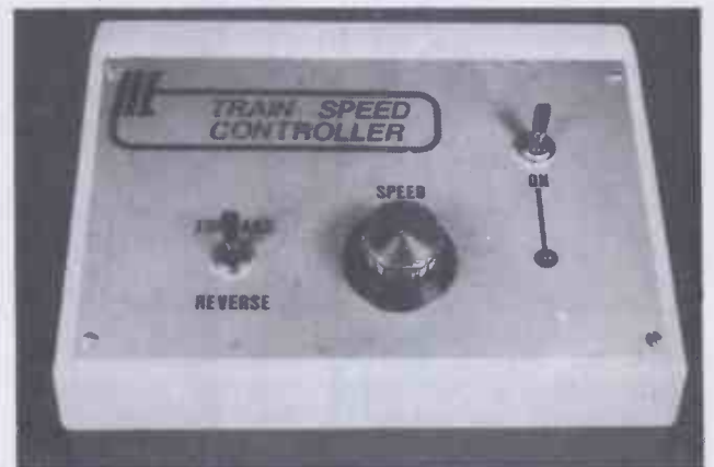
Our prototype train controller built in a Verobox. It cannot be seen from this photograph but holes should be drilled into the case to provide adequate ventilation otherwise the heat buildup can cause the safety cut-out thermistor to trip.
