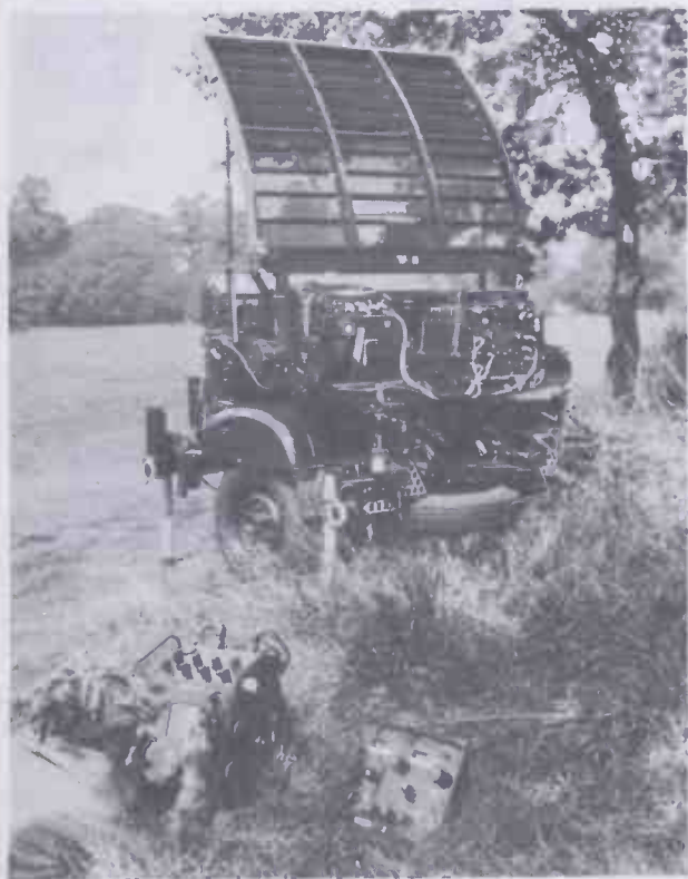
CYMBALINE anti-mortar radar. By hitting the projectile with a radar beam at two points on its flightpath the unit is able to 'project back' the firing position. This enables the operator to 'call down' fire upon the enemy's head with great accuracy. CYMBALINE is light enough to be removed from its trolley and comfortably carried by four men.
