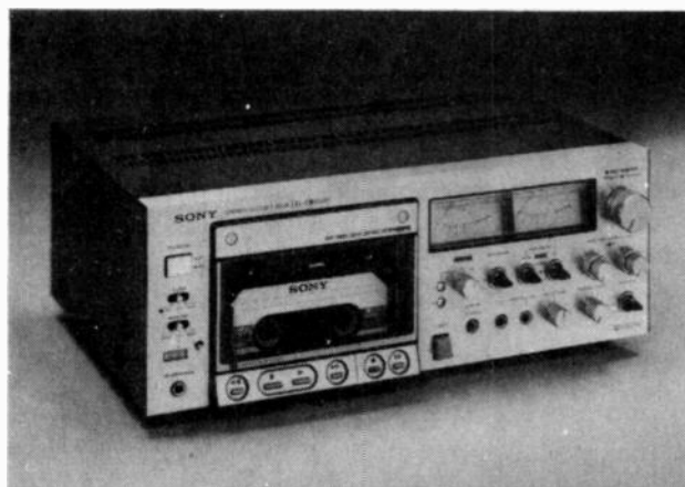
Sony's excellent EL7 recorder. Conceived as a cassette tape machine which would have open-reel performance (by using tape at a higher speed basically) even if it is dependent upon those bias switches to optimise performance.
