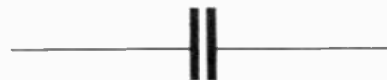
Fig. 2. Symbol for a capacitor. This symbol is used for a fixed capacitor, meaning a capacitor whose value is not deliberately changed (as for tuning a radio). A slightly different symbol is used for an electrolytic capacitor.
