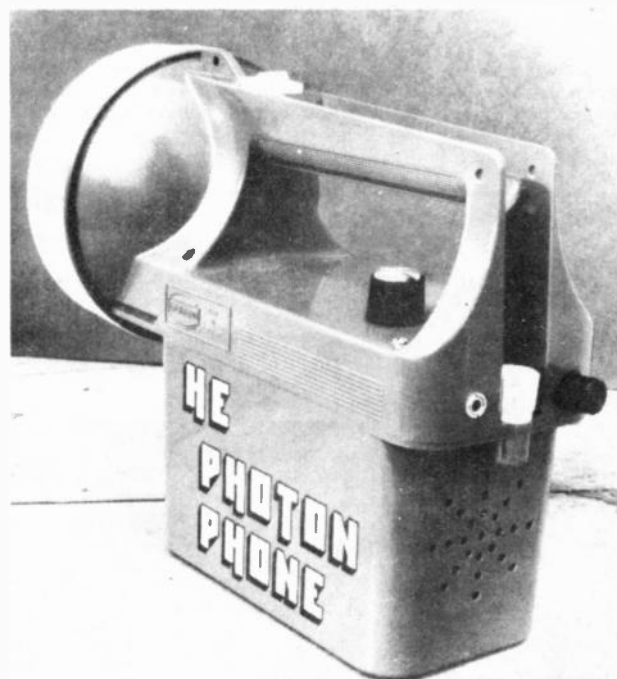
A rear view of the PHOTON, showing the artistic pattern of holes we drilled to form the speaker grille!
