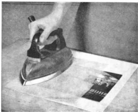
The picture has been laid in position on the mount, covered with grease-proof paper and the iron applied
