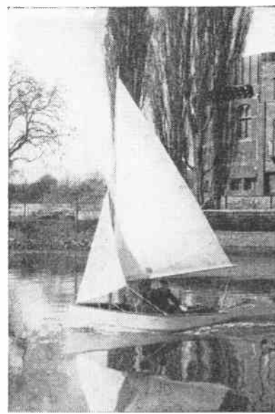
The 'Wensum' dinghy sailing under gunter sloop rig. A suit of sails can be bought for £10-£15, or can be made by the sailing enthusiast himself.
