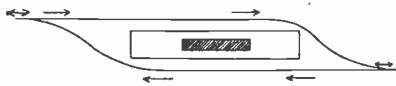
Fig. 1—Simple single-line passing station advantage of the facility offered by the 'unit' type of track for quick experiment, it is a good idea to get to understand how the various standard track units—the straights, half-straights, the curves and the turnouts—can be best incorporated into any layout design to produce the best and most workable plan. It is then quite an easy matter to fix the track permanently to the baseboard if so desired to produce a real 'permanent way'.
