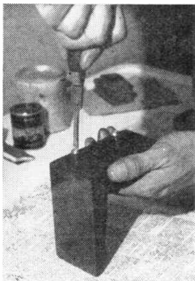
Fig. 3—Screws being fitted into the back of the finished pattern for bookends to assist in removing it from the mould
