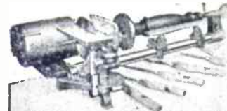
Showing arrangement for turning between centres and sawing.
