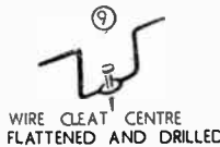
CLEATS. DRILL HOLES AND FILE TO SHAPE
