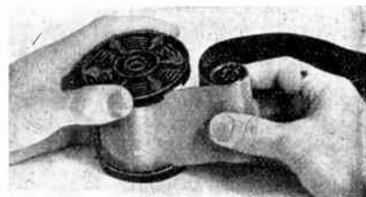
Loading the film into the tank
