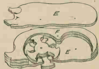
Fig. 4—The "walking" mechanism in position
