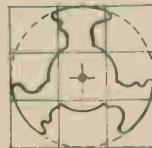
Fig. 5—How the leg pieces are marked out and cut.
