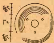
Fig. 7 (right)— Section of earphone and view showing drill holes
