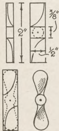
Fig. 3 Details of the propeller
